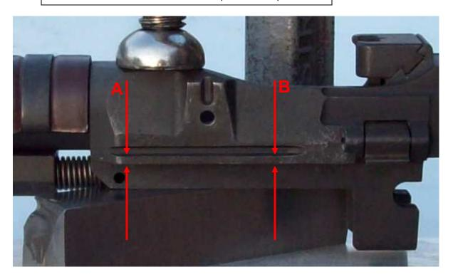
Second: find a flat steel surface to place against the base of the action as well as log steel rod or surface that should run the length of the barrel and clamp it all together.
