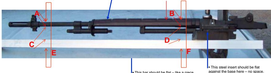
OR Measure A and B, and then measure from the top of the barrel to the bottom of the steel rod or object that is parallel with the action for measurement E and F.
